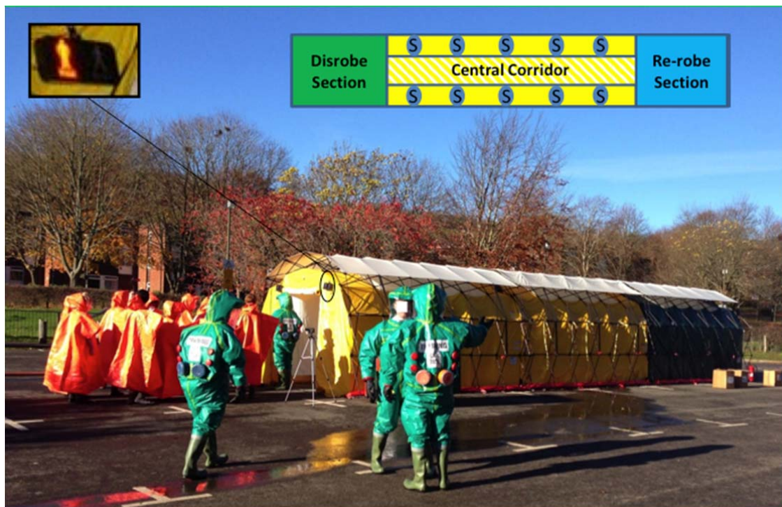
Figure 7: Mass casualty decontamination unit (“MDI”) deployed by UK specialist responders. Photograph acquired during an exercise and shows a group of 10 individuals in high visibility ponchos (from “disrobe packs”) waiting to enter the unit in accordance with a “traffic light” system (inset, top left). A schematic of the unit (inset, top right) indicates position of disrobe area, two side corridors (each with five shower areas [“S”] for decontamination of ambulant casualties) and a central corridor (used by responders to observe or instruct individuals) which can be adapted for processing non-ambulant casualties. Air heaters and a boiler for shower water are at the rear of the tent and so not shown in this image. Reproduced with permission of Public Health England ©2013.
