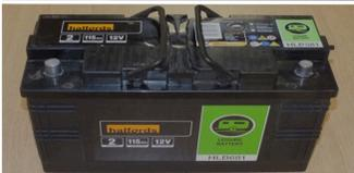
Battery. This 12v lead-acid battery can power the tool for 8-9 hours.
