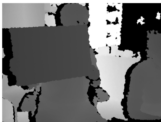
Figure 3. Kinect sensor depth image. The sensor produced this depth image from the infrared (IR) dot image in Figure 2.
