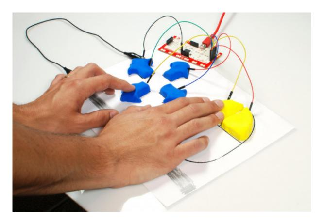
(Hint: Get creative with the ground connection. In the example above, we connected ground to a penciled bar where we rested our hand.)
