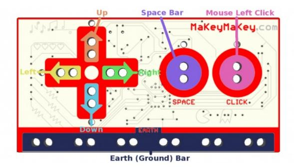
Each of those inputs as well as the very important "Earth bar" are available in the form of what I like to call "alligator-bait" connectors. You'll use the included <u>alligator clip cables</u> to clip right into the hole pairs. This will all be made much more clear in the next section. For now, let's keep summarizing your MaKey MaKey.
