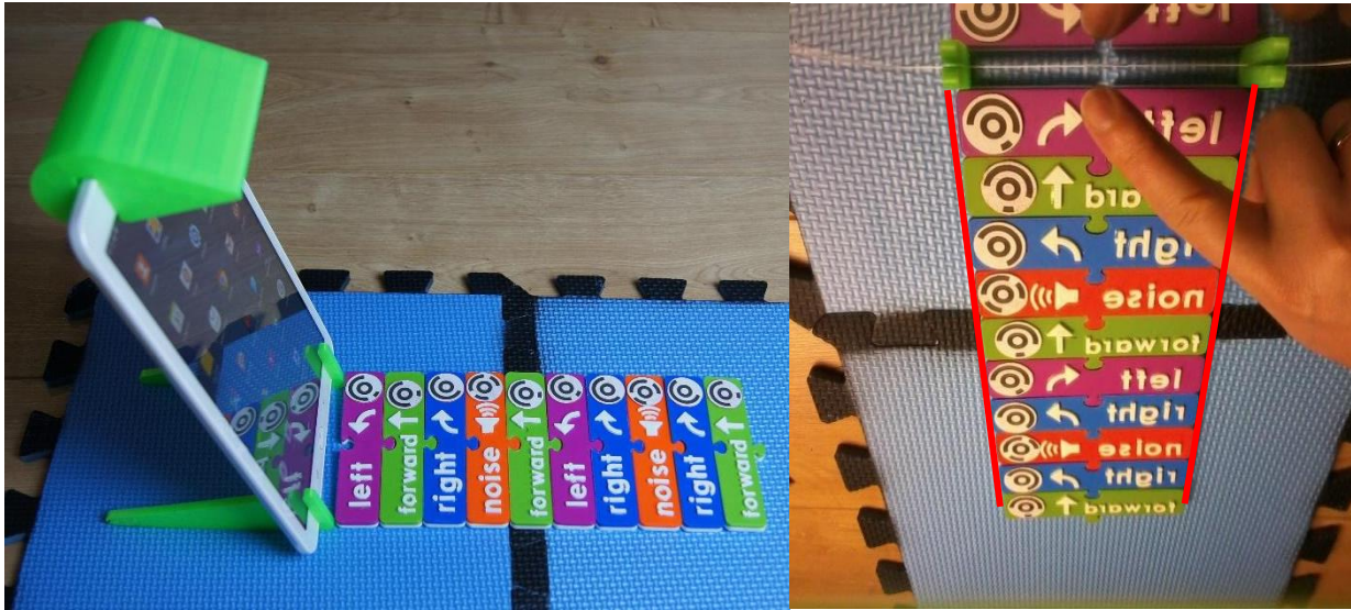
Figure 70: Original stand angle and resulting image with distortion of codes
