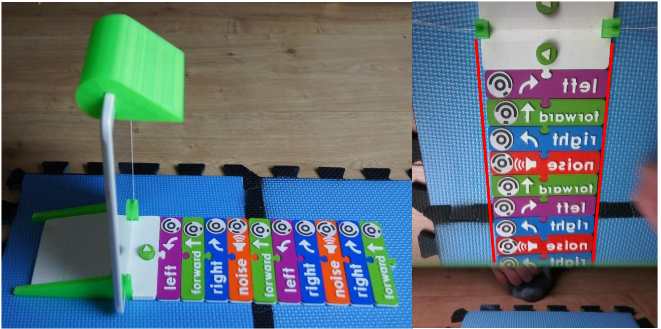
Figure 72: Upright stand angle and resulting effect on captured image.
