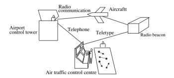
Fig. 6. First generation air traffic control system (Gilbert, 1973, p. 97).
