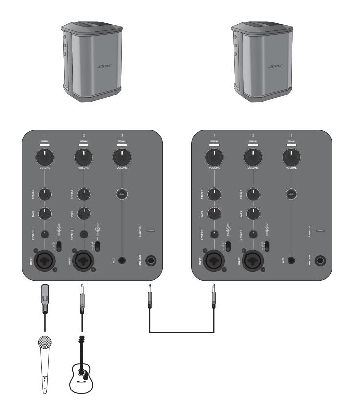
**Note:** On secondary units, set ToneMatch<sup>®</sup> and reverb to off and leave tone controls at center detent position.
