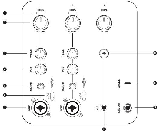
Use Channel 1 and 2 inputs for microphones and musical instruments. Integrated ToneMatch<sup>®</sup> signal processing allows microphones and instruments to sound their best. Use Channel 3 for *Bluetooth*<sup>®</sup> connectivity and line-level inputs.
