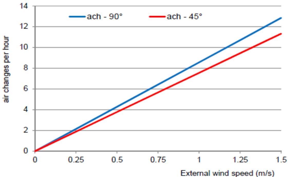
This demonstrates how effective natural ventilation via open windows is. CIBSE have made assumptions for the calculations, for instance “a coefficient of discharge (Cd) of 0.61 is adopted based on cl 4.6.1 of CIBSE Guide A to take into account the pressure drop through a sharp edged opening, such as a window. The resulting air flow rates are shown in Table 5.”
