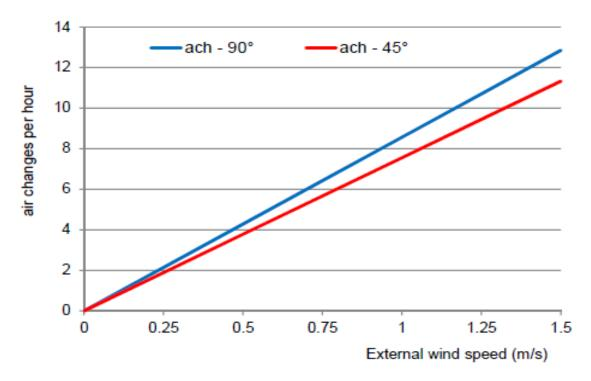
This demonstrates how effective natural ventilation via open windows is. CIBSE have made assumptions for the calculations, for instance "a coefficient of discharge (Cd) of 0.61 is adopted based on cl 4.6.1 of CIBSE Guide A to take into account the pressure drop through a sharp edged opening, such as a window. The resulting air flow rates are shown in Table 5."
