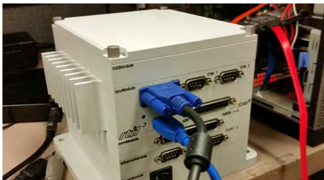
The second version of the Advanced Scalable Assured Positioning, Navigation and Timing (ASAP) system prototype, which is roughly half the size of a shoe box. Photo by Michael Ferguson
