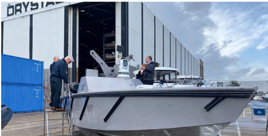
One of the unmanned surface vehicles used in the test included the British 9-meter Maritime Autonomy Surface Testbed vessel. Photo courtesy of Christian Schumacher
