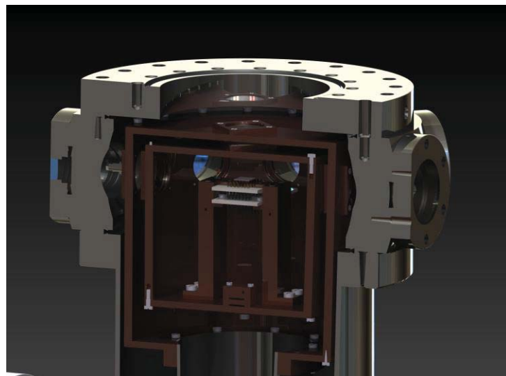
Figure 1. Cross section of the microtrap in the cryo-system.
