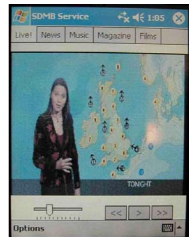
Figure 1: Demonstrator for mobile TV with channel tabs on top, play/pause, skip buttons, and audio control on the bottom
