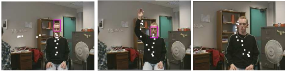
(a) System responding to a waving gesture by zooming in on the subject.
