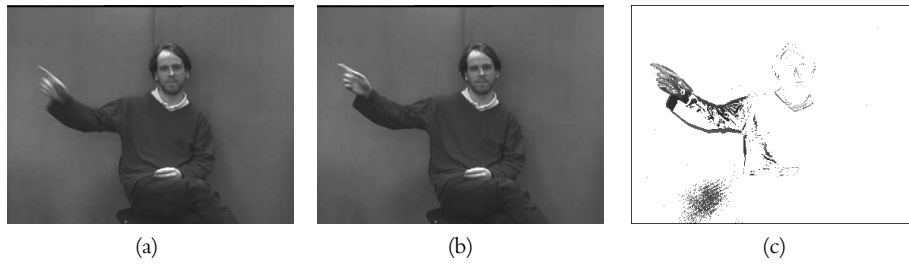
Fig. 2. Example of differencing two consecutive frames (a) and (b), result in (c), from a ‘point with the right hand to the right’ ( pntrr ) gesture.
