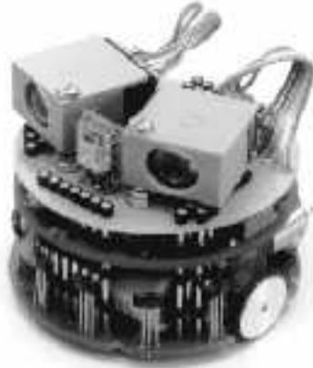
Figure 2: The Khepera mobot (from the K-team WWW pages).
