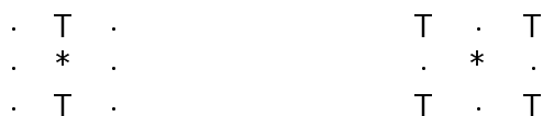
Figure 14: Aliased sensory input in woods102 : the input pattern on the left occurs in four cells (labels 4, 5, 17, and 18); the input pattern on the right occurs in two cells (labels 2 and 15). For both patterns, different appropriate actions are required at the different cells.
