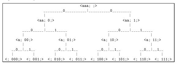
A node in the tree is represented by a two-argument list of the form *distance list*; *label*; , where the distance list is a sequence of a's whose length is the distance to a terminal node, and the label on the node is the concatenation of the edge labels up to the root. Left branches are labelled with 0, right branches with 1.
