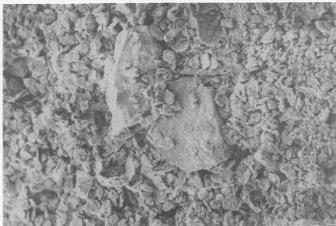
Figure 1a. Grains from a Group 1 sample; clean faces, clearly defined grains. (x500; 1cm = 10 \mu m)
