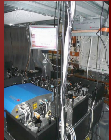
Lasers & Optics required to cool single charged atoms close to absolute zero. (~-273°C)
