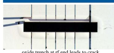
Electrode breakage generally is low. An asymmetry of shear stress at RF electrode end appears to lead to cracking. Avoiding this asymmetry eliminates fractures.
