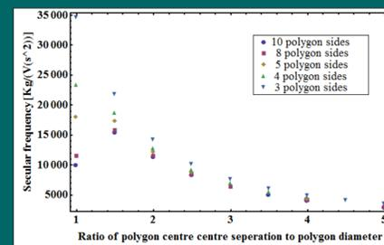
Right shows the secular frequency of the ions against polygon separation, A, given as a ratio of the separation to the polygon diameter. The polygon diameter was kept constant at D = 400  $\mu$ m.
