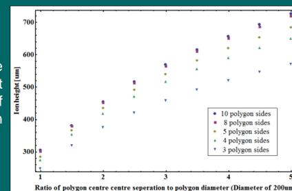
Right shows the height of the rf nil about the surface of the polygon array, h, against polygon separation, A, given as a ratio of separation to polygon diameter. The polygon diameter was kept constant at D = 400  $\mu$ m.
