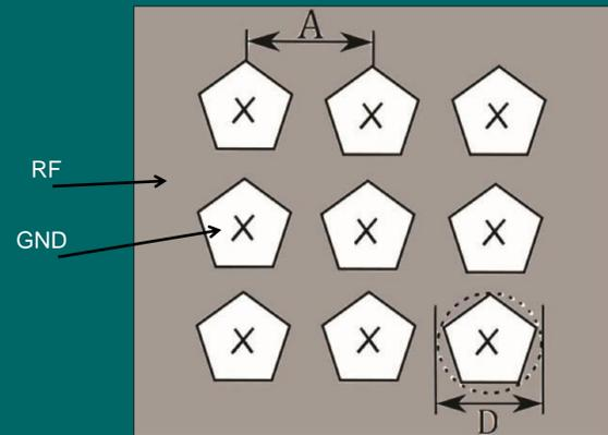
By controlling the number of sides of each polygon, the diameter of the polygon, D, and the ion-ion separation, A, optimisation of the trap parameters and quantum simulator suitability can be achieved.
