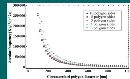
Left shows the radial secular frequency of the trapped ions against the polygon diameter, D. The polygon separation was kept constant at  $\frac{5}{4}D$ .
