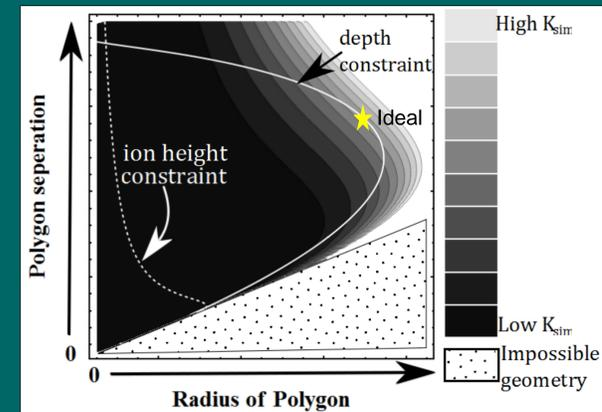
For <sup>171</sup>Yb<sup>+</sup> with an rf amplitude of 200 V at 15 MHz drive frequency, the trap depth, secular frequency and  $K_{sim}$  were then calculated in an 11x11 array.
