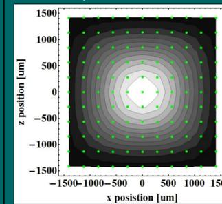
Left shows a  $K_{sim}/F^2$  contour plot with contour lines of  $0.5 \times 10^{36} N^{-2}$  up to  $6 \times 10^{36} N^{-2}$ . The ions are marked by a green dot. Bottom left shows trap depth contours of 0.05eV up to 0.5eV at the edge. Bottom right shows secular frequency contours of 0.1MHz up to 1.5MHz at the edge.
