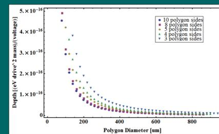
Left shows the trap depth against the polygon diameter, D. The polygon separation was kept constant at  $\frac{5}{4}D$ .
