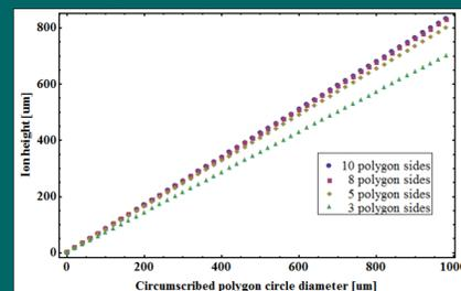
Left shows the height of the rf nil above the surface of the polygon array, h, against the circumscribed diameter of the polygon, D. This was repeated for several different polygon side numbers, n. The polygon separation, A, was kept constant at  $\frac{5}{4}D$ .
