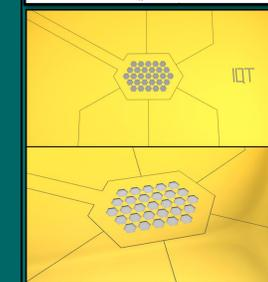
Left shows drawings of the proposed ion trap lattice. It comprises of 29 trap sights and is surrounded by 6 compensation electrodes. Below shows the trap lattice during fabrication, the grey hexagons are the exposed top silicon layer, before they are etched away.
