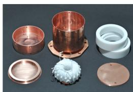
toroidal superconducting resonator
