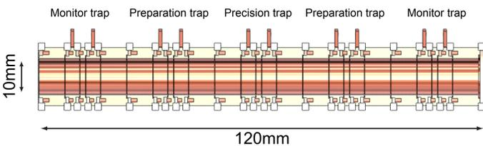
The PENTATRAP-tower consists of five identical cylindrical open-endcap Penning traps. The inner diameter is 10mm and the length of a single trap is 24mm. The five-pole structure of each trap allows for compensation of electrostatic anharmonicities. Therefore, the axial frequencies are independent on the ion's energy, which is crucial for high-precision experiments where tiny frequency shifts have to be detected. The most important design criteria are listed below:
