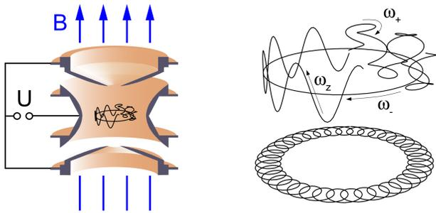
A charged particle confined in a superposition of a strong homogeneous magnetic field  $B$  and a weak harmonic electric field supplied by voltages  $U$  at the trap electrodes, performs three independent eigenmotions:
