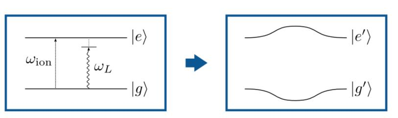
In a dressed atom picture, the potential can be identified with the positiondependent energy shift of the atomic levels.
