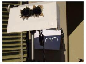
Take care that the binoculars are not pointing at the Sun for too long, as this may damage them. This should not be a problem if the binoculars are on a static mount, which does not track the Sun. The Earth rotates such that the Sun appears to move across the sky by its own diameter (0.5 degrees) in just 2 minutes, so the binoculars will need to be repointed every few minutes to follow the Sun which could damage the binoculars if they are not filtered.
