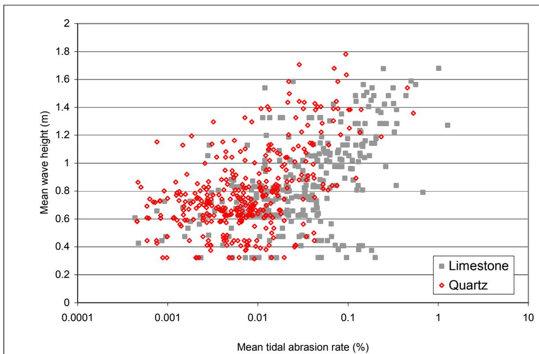
Figure 28: Mean tidal abrasion rate in relation to mean wave height for 681 pebbles.
