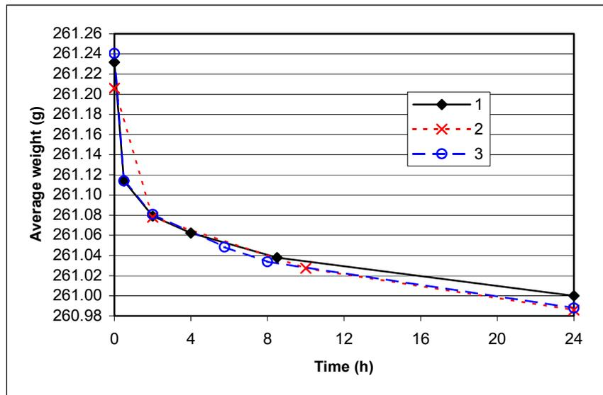
Figure 16: Average weight change of 15 flint pebbles after 24 hours of wetting and 24 hours of drying at 50°C. The initial weight at room temperature was 261.072 g. Curves 1 to 3 show three successive drying cycles.
