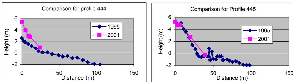
Figure 37: Comparison of profile data for the two profiles of the beach between Telscombe Treatment works and Saltdean. Profile 1995 from EA data, profile 2001 from terrestrial survey.
