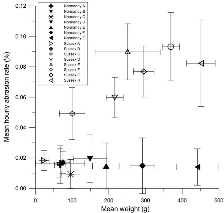
Figure 17: Comparison of abrasion rates between flints from East Sussex and Normandy in relation to size (weight). Error bars are 1 standard deviation.
