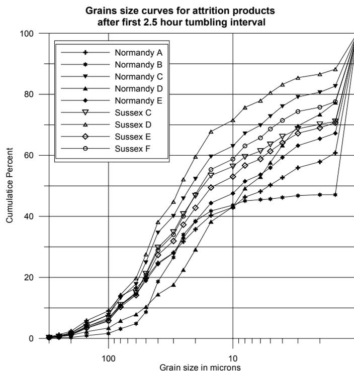
Figure 18: Comparison of grain size of the abrasion products after the first 2.5 hours tumbling interval.
