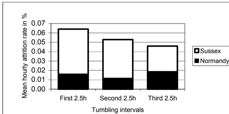
Figure 19: Abrasion rates for three successive tumbling intervals of 2.5 hours each, averaged over all samples from Normandy and Sussex included in the main experiments
