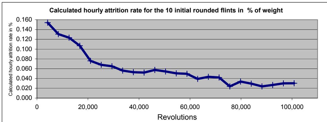
Figure 13: Averaged mean hourly abrasion rate for the 10 pebbles starting the experiment.
