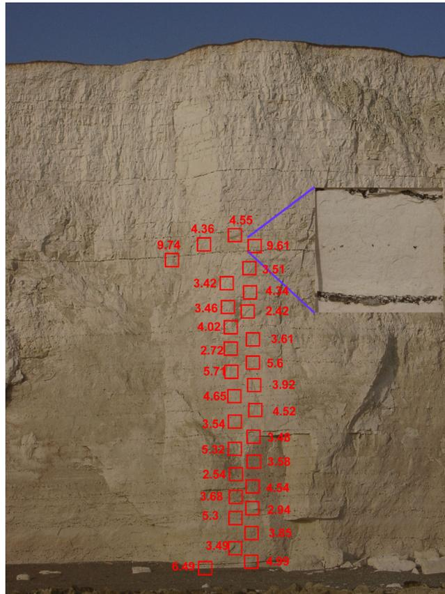
Figure 8: Overview of flint content for Belle Tout beds in the lower Seaford Chalk east of Birling Gap. Inset image shows the Seven Sisters flint band.
