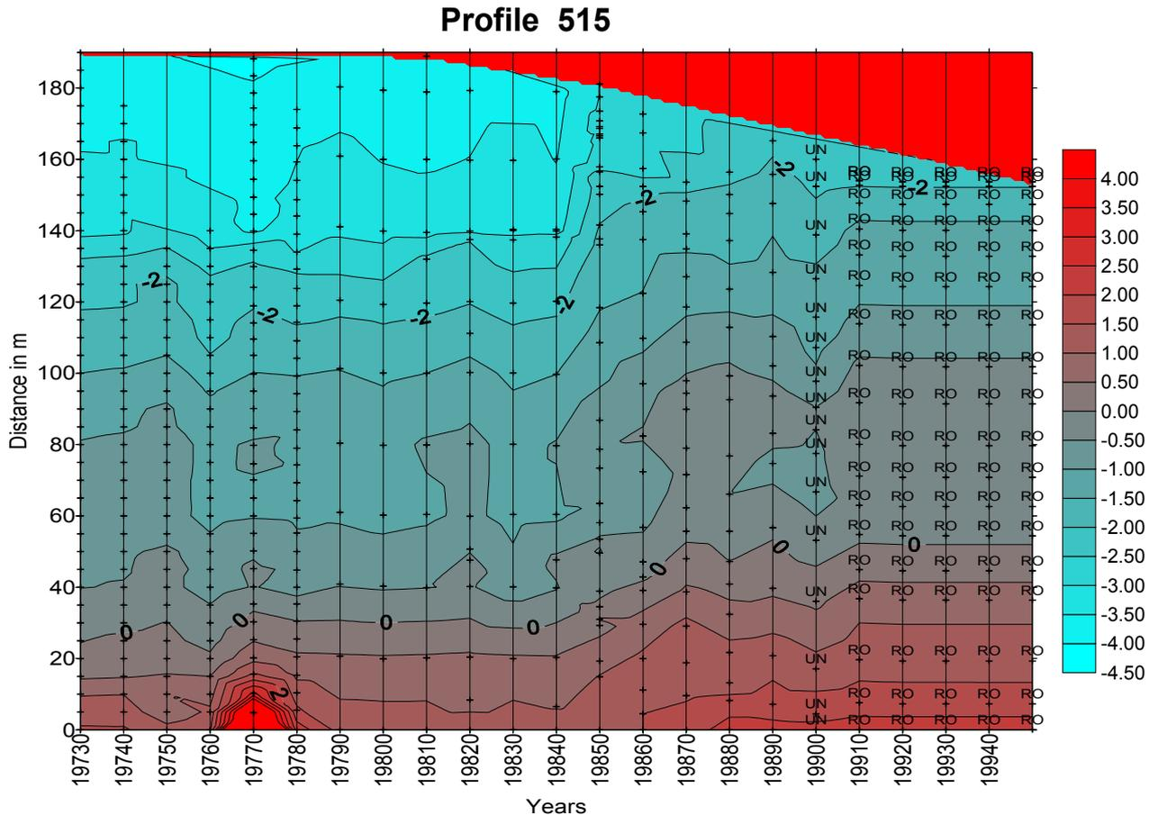
Figure 34: Graphs showing the surface elevation of profile G515 in front of the Belle Tout lighthouse for the years 1975 to 1995
