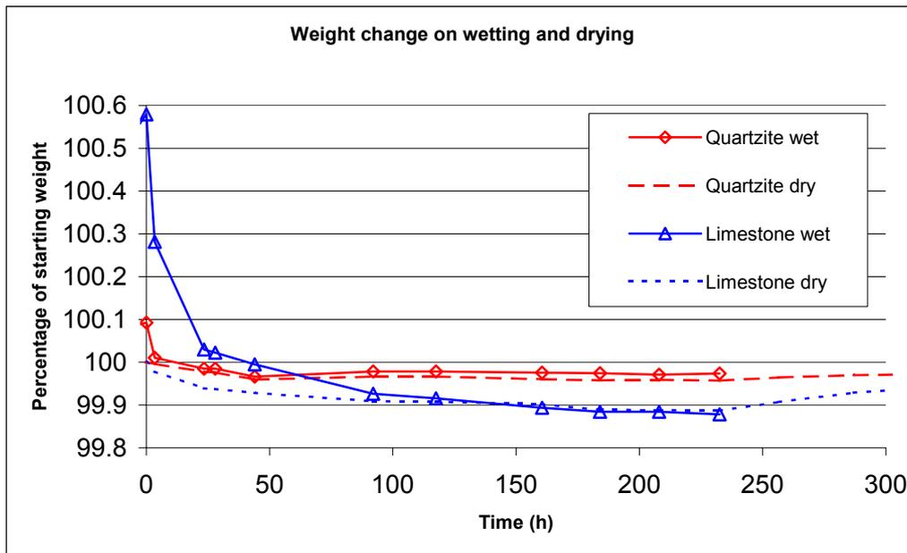
Figure 24: Weight changes for 10 limestones and 10 quartzites.
