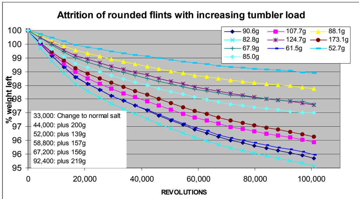
Figure 11: Change of abrasion rate with a gradual increase in the tumbler load. Abrasion of individual pebbles decreases with the time.
