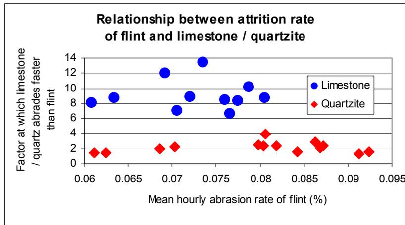
Figure 31: Abrasion rate of 11 limestones and 14 quartzites in relation to the abrasion rate of flint.
