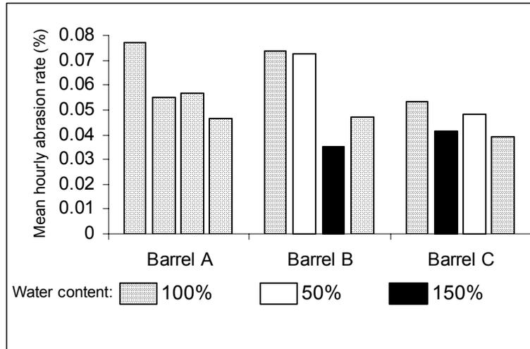
Figure 15: Mean hourly abrasion rate for a random samples of beach flint from Telscombe. Barrels were filled to 33% with pebbles, water content varied between 50 and 150%.
