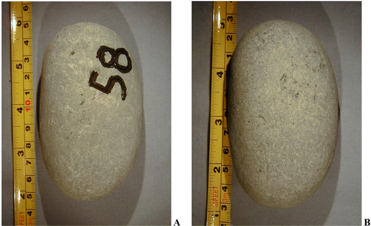
Figure 23: Limestone pebble no 58 (354.92g in A) lost 5.3% of its weight (B) during 5 tides on Saltdean beach in April 2001 (mean wave height 1.7m).
