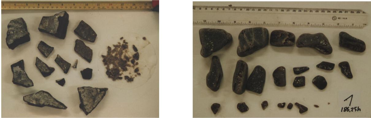
Figure 10: Abrasion of freshly broken flint after 0.15 and 186.15 hours of tumbling.
