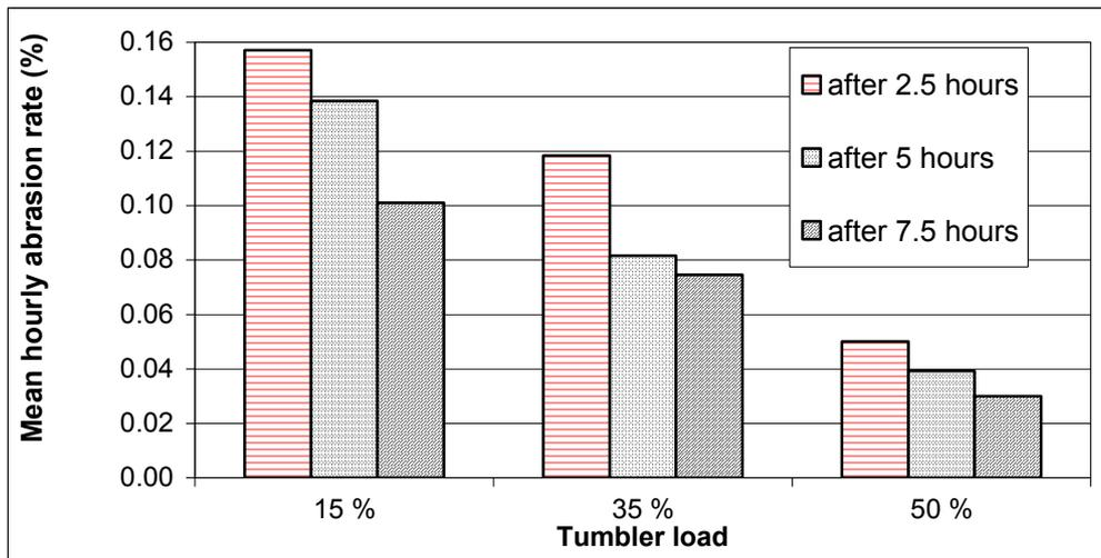
Figure 14: Mean hourly abrasion rates expressed as %weight loss for three different barrel loads and three successive tumbling intervals each of 2.5 hours duration.
