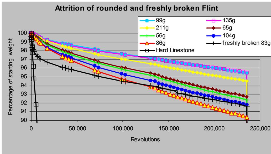
Figure 9: Graph showing the wear of nine flints in relation to tumbling time and tumbling interval. The slight change in abrasion rate at 132 hours is due to a balance error. The hard limestone abrades extremely quick in comparison and was removed after 10,000 revolutions.
