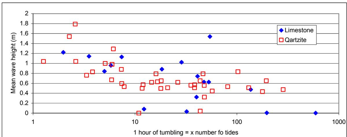
Figure 33: Comparison between field and tumbler abrasion rates.
