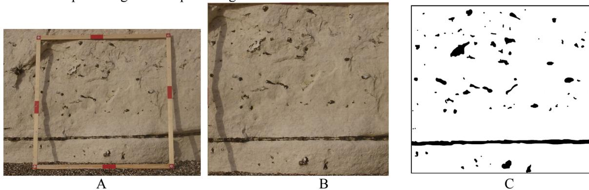
Figure 7: Process steps for calculating flint content in Chalk (flint content for this 4m<sup>2</sup> section is 4.9%).
