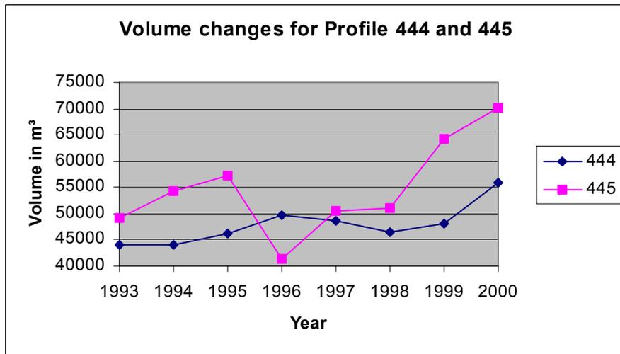
Figure 38: Volume changes for the two profiles of the beach between Telscombe Treatment works and Saltdean.
