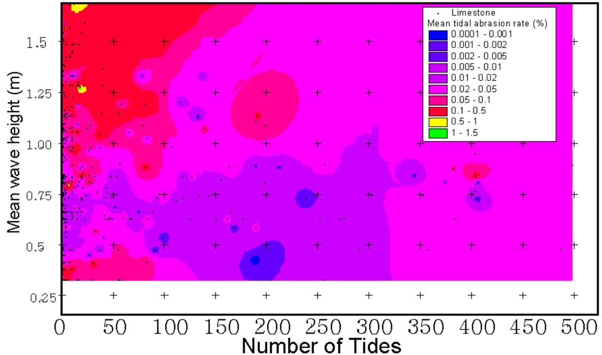
Figure 30: Abrasion rate for limestone in relation to mean wave height and the number of tides.
