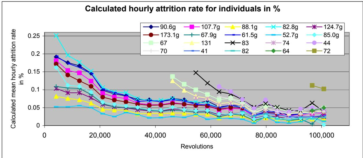
Figure 12: Individual curves for the change in abrasion rate of the 10 initial pebbles shown in figure 11 and those added at intervals.
