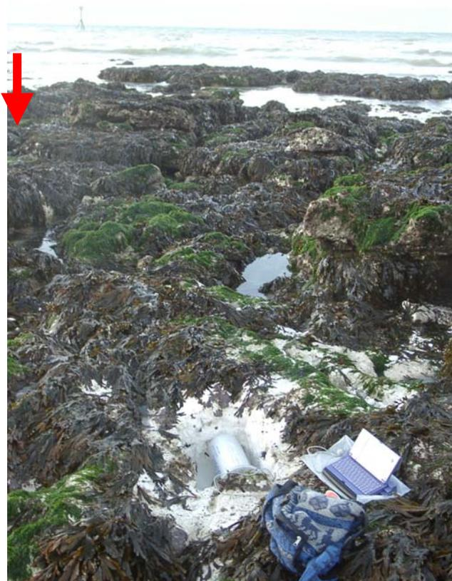
Figure 1: **Telscombe**. A hole measuring 30cm x 50cm and 25 cm deep was excavated into the platform which took  $x = 539146.931$ ,  $y = 101391.797$  and  $z = -1.482$ m OD. The recorder is 39m seawards of the beach toe and 80m seawards of the cliffs backing the beach. The recorder was always submerged in the hole, providing a rather stable pressure when the tide was not covering the recorder. The red arrow shows the location where the MIDAS directional wave recorder was placed.
