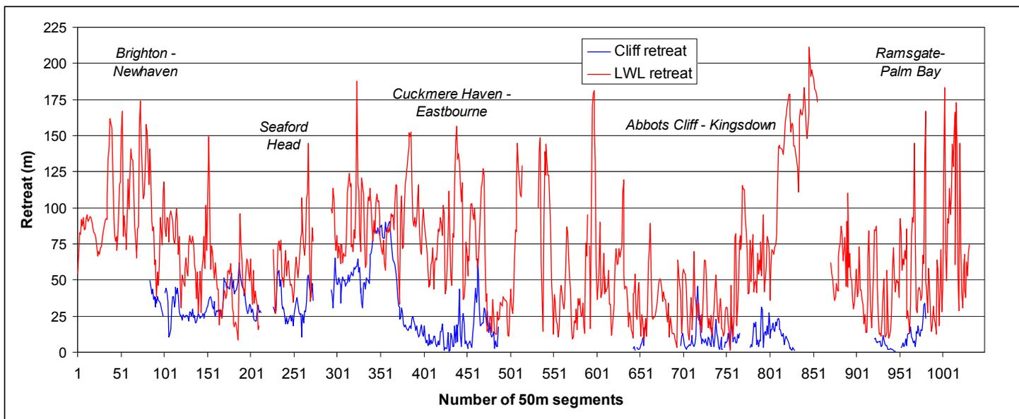
Figure 5: Retreat of the LWL position between the 1<sup>st</sup> Edition Ordnance Survey maps (surveyed in the 1870s) and the landline data (about 1990s). For comparison the retreat of the cliff for the same period is shown. Gaps between sections of the coast not to scale.
