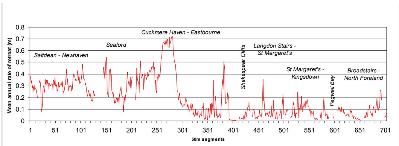
Figure 3: Mean annual rate of chalk cliff retreat along the East Sussex and Kent frontage for the period 1870s to 2001. Names refer to the start and end point of the cliff section; gaps between sections not to scale.
