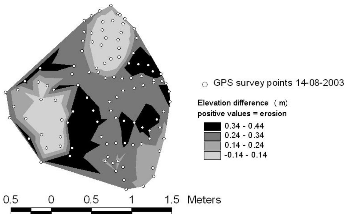
Figure 7: Comparison between GPS points surveyed on 14-08-2003 and DEM generated from air photo flown on 05-05-2001. DEM resolution is 10cm. The comparison shows two areas remaining at the same elevation in 2003 as in 2001 (light grey) with the chalk between eroded which is the same situation as shown in fig 7.
