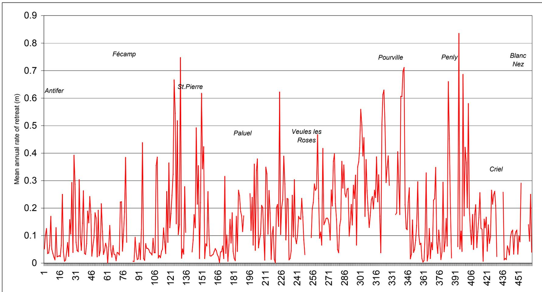
Figure 4: Mean annual rate of chalk cliff retreat along the French coast 1966 to 1995 (1944 to 1999 at Cap Blanc Nez, Lahousse et al 2000). Names refer to locations between cliffed sections; gaps between sections not to scale.
