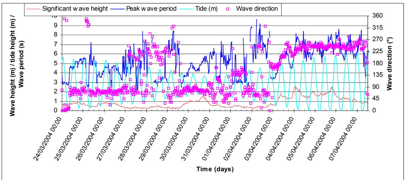
Figure 26: Wave conditions at the Hastings buoy and tidal predictions for Newhaven (heights only as a relative indicator of the state of the tide).
