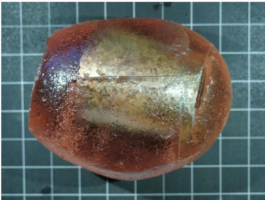
Figure 29: Crack and cavity of pebble 248
