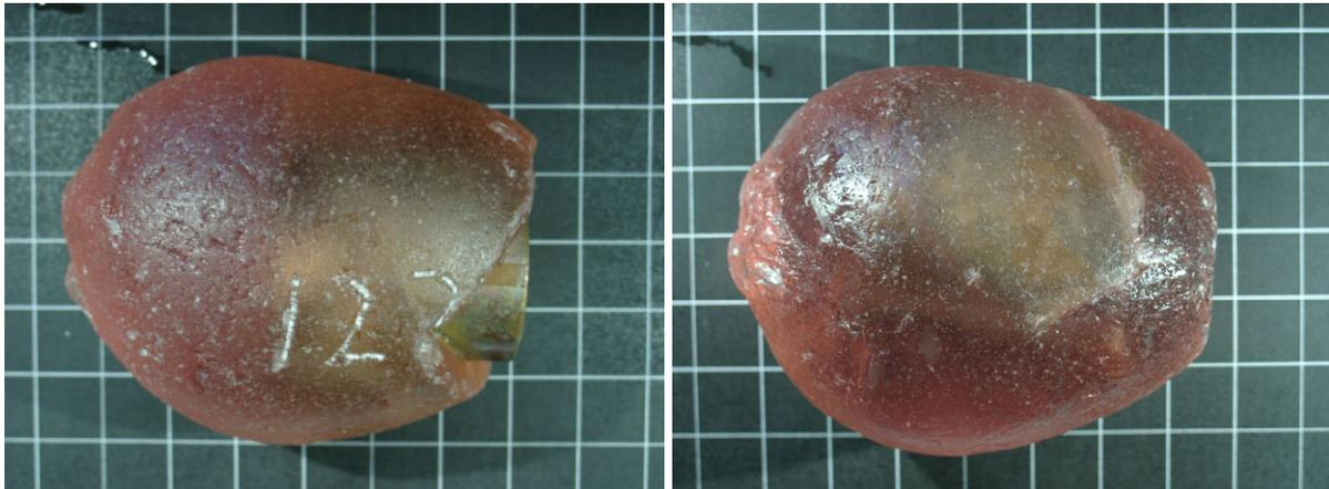
Figure 20: Examples of broken (left) and cracked (right) tracers found on 12-03-2004.
