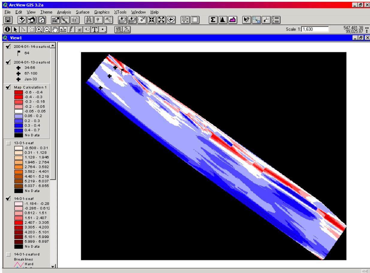
Figure 11: Comparison of surveys at Seaford. Black crosses show deployment points, black flag shows the position of the relocated pebble. Blue shows accretion, red erosion, though some of the erosion on the higher part of the beach is due to survey error.
