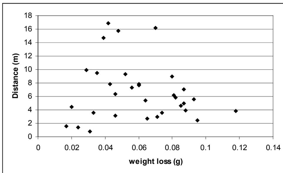
Figure 30: Scatter graph of distance the tracer moved from its deployment point in relation to the absolute weight loss.
