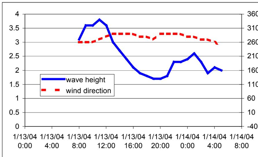
Figure 9: Wave and wind condition at the Greenwich light ship (~50km south of Newhaven).
