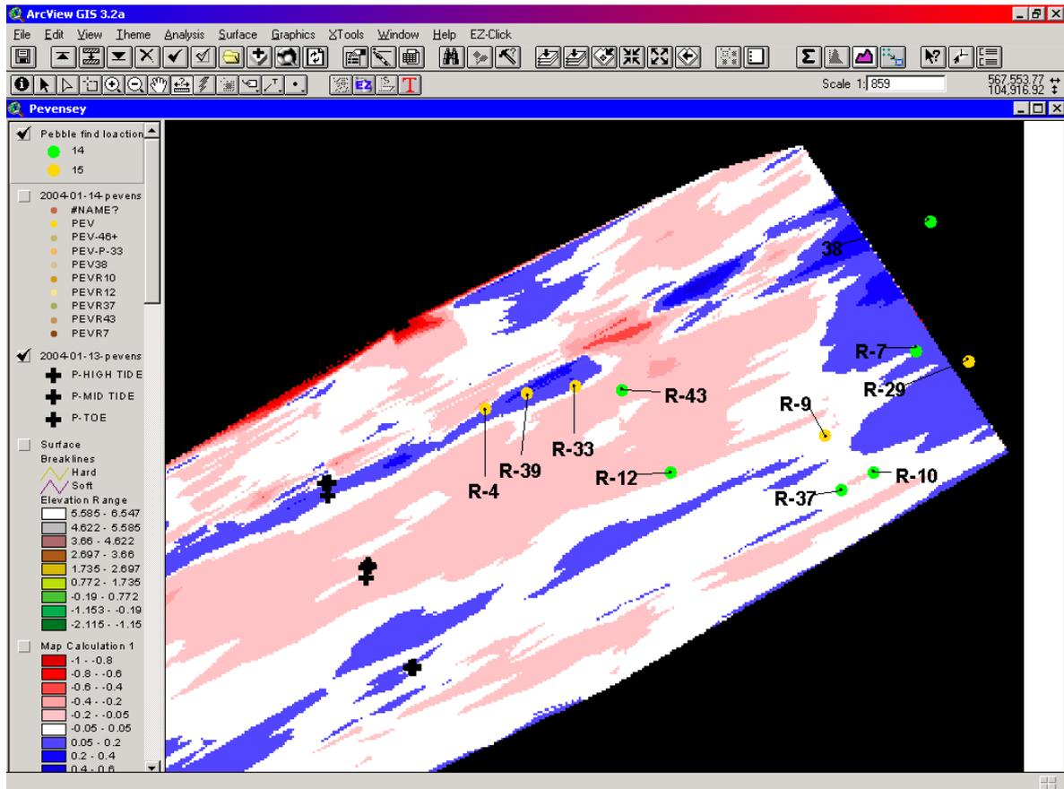
Figure 14: Difference in beach elevation between 13-01 and 14-01. Black crosses are deployment points. Green dots show locations of pebbles found on 14-01, yellow dots those found on 15-01; R denotes resin pebble.
