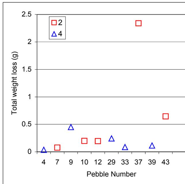
Figure 15: Total weight loss of the 10 resin pebbles from January 13 to 15, 2004. Red squares indicated recovery after 2 tides, blue triangles after 4 tides. Exceptional weight loss of 2.3g is due to breakage.
