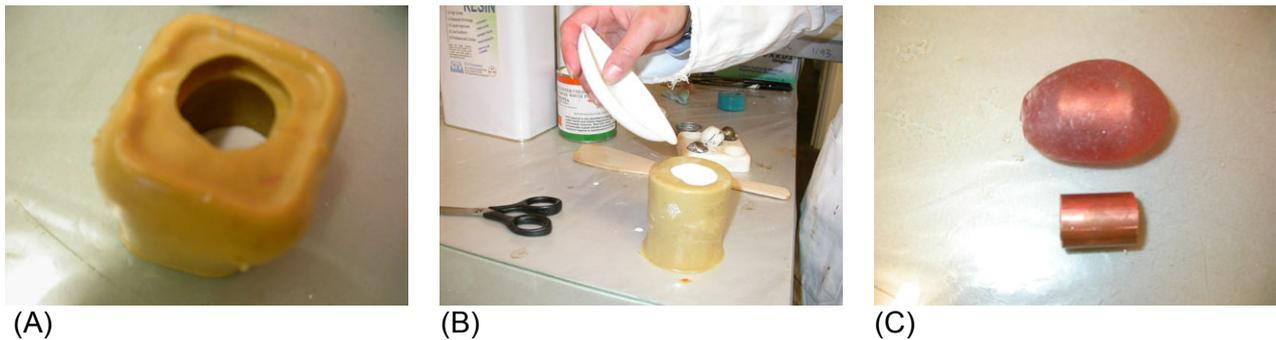
Figure 4: Manufacturing resin pebbles.
