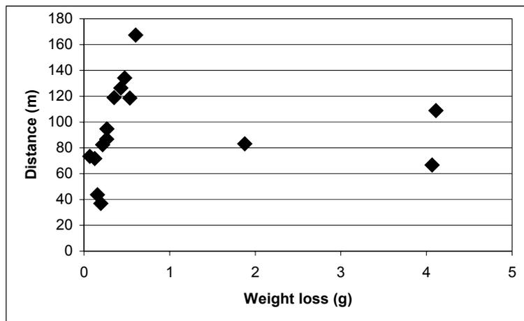
Figure 21: Scatter graph of distance the tracer has moved from its deployment point in relation to the absolute weight loss (Only cracked or intact tracers were considered).
