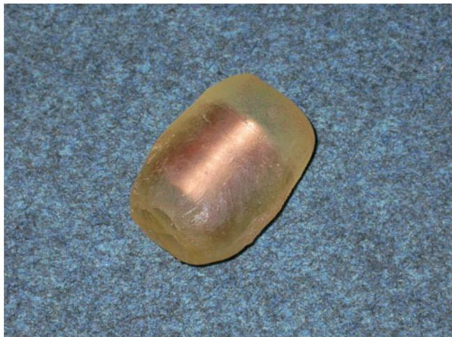
Figure 7: Final resin tracer pebble
