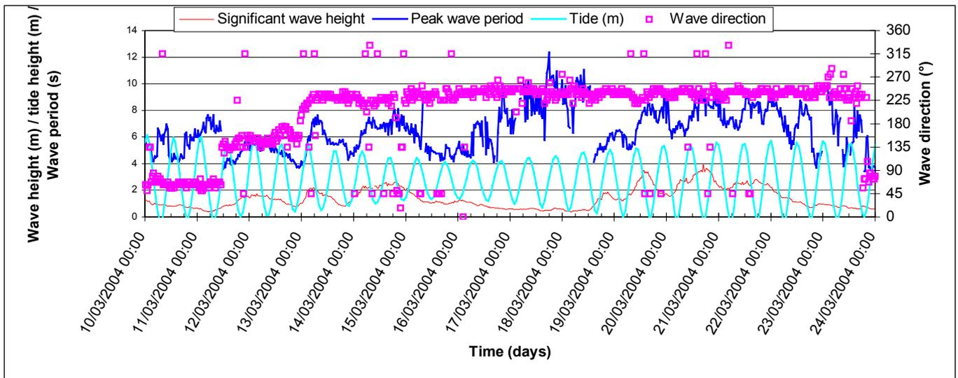
Figure 18: Wave conditions at the Hastings buoy and tidal predictions for Newhaven (heights only as a relative indicator of the state of the tide).
