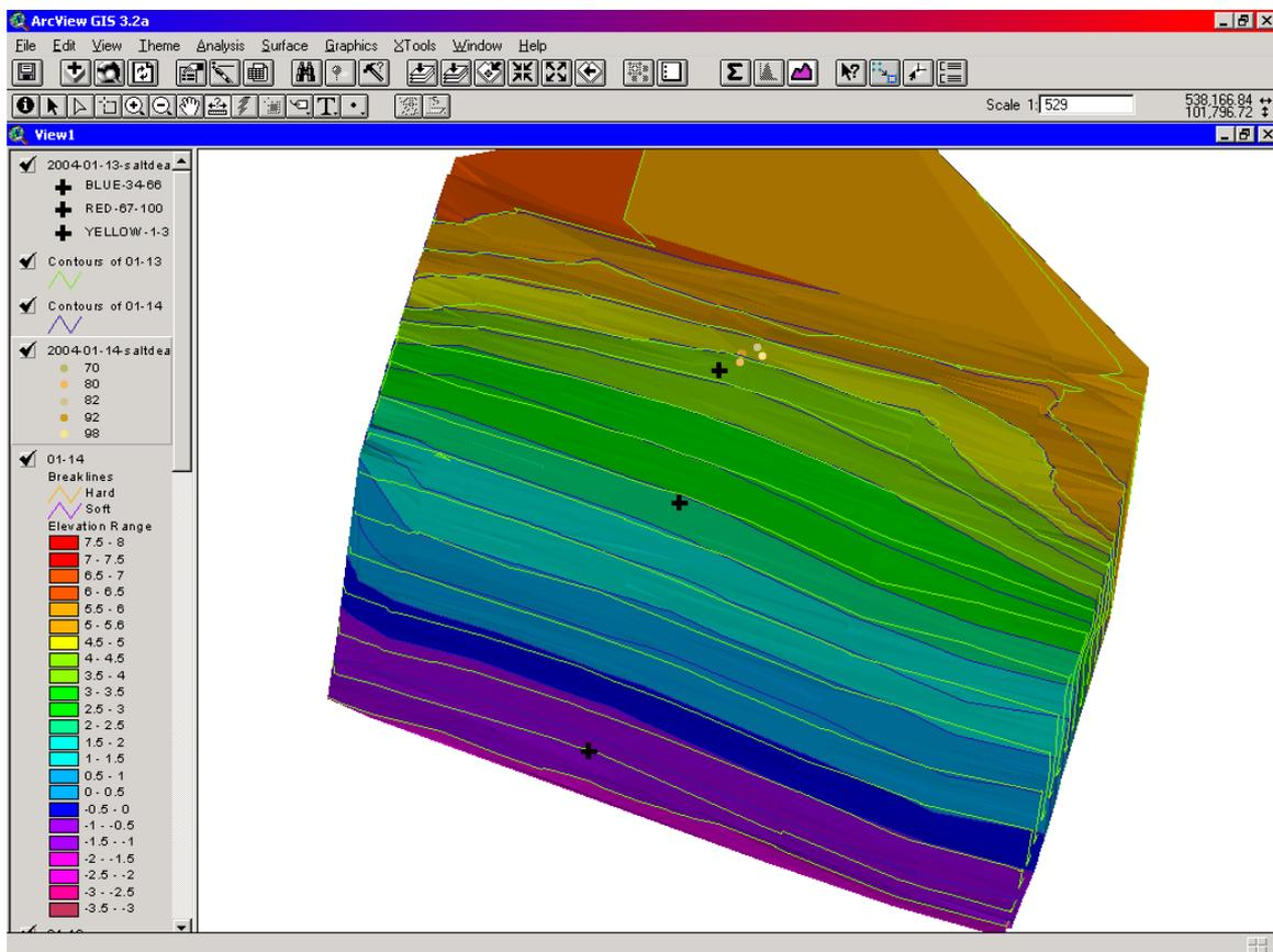
Figure 10: Black crosses show deployment points and light brown coloured dots the positions of relocated pebbles. Contour lines for both surveys are overlaid over the surface of the 14-01-2004.
