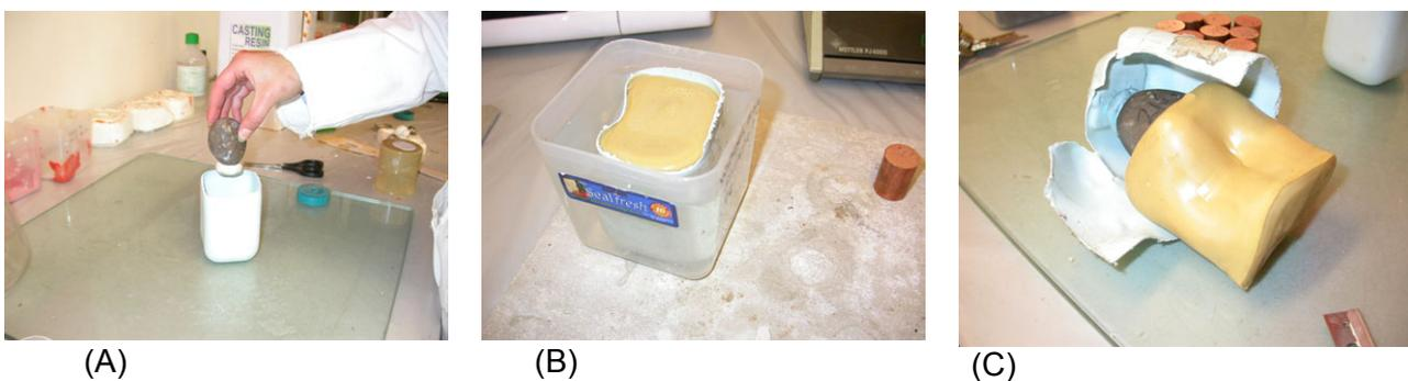
Figure 3: Manufacturing resin pebble moulds
