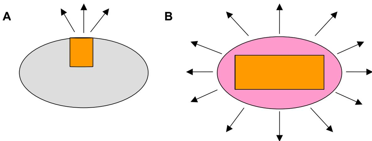
Figure 2: Drilled flint (A) allows for the insertion of only a small metal rod, manufacturing resin pebbles (B) allows a large metal core to be embedded maximising cross-sectional interference.
