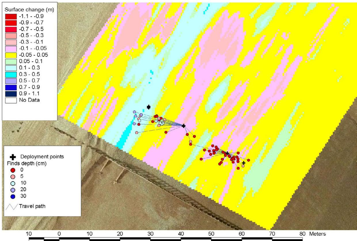
Figure 28: Detailed diagram of recovery locations and surface change on 26-03-2004.
