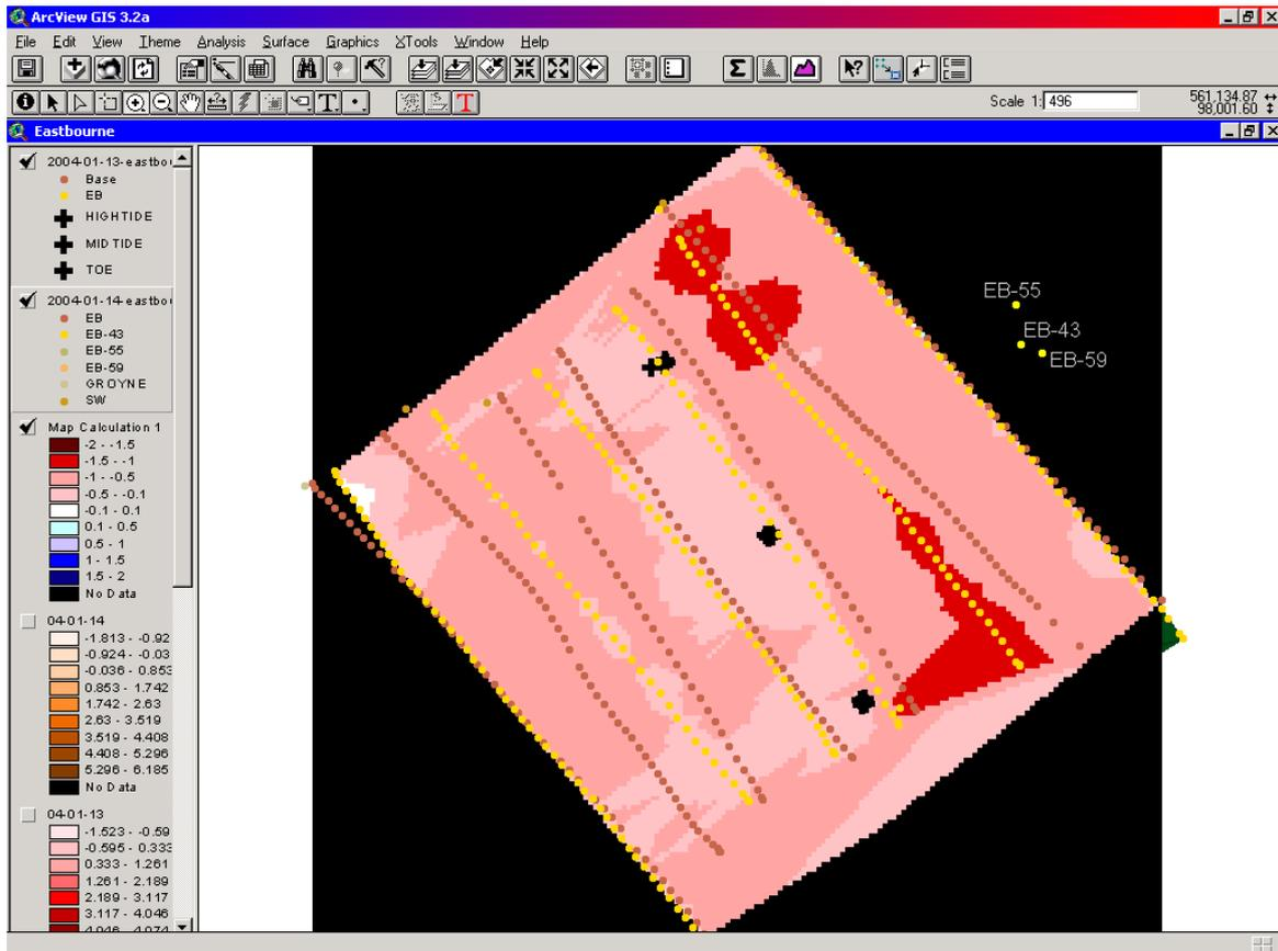
Figure 12: Comparison of the surveys at Eastbourne showing the difference in height between the two surveys. Black crosses show deployment points, yellow dots with label show location of found painted pebbles. Groyne compartment width is 59m.
