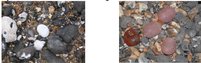
Figure 1: Pictures of both tracers used to investigate the longshore transport. A-Picture of a new natural tracer. B-Picture of the resin cobbles.
