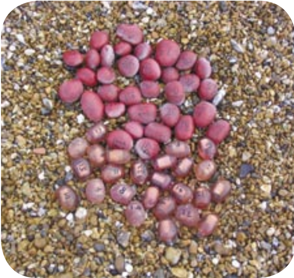
Deployment of painted and synthetic tracer pebbles at Pevensy Bay beach.
