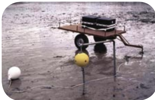
Deployment of fluorescent sand tracer (A) and current meter (B) on the Sainte-Marguerite-sur-Mer Beach.
