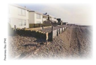
Whilst erosion of the chalk adds some new flint to our beaches, BEACHES AT RISK has calculated that this is just a fraction of what is lost through shingle wear and longshore drift.
