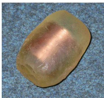
A synthetic tracer pebble, as used in the BAR experiments. Notice copper core inside pebble.
