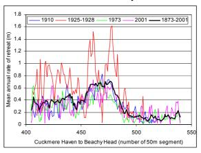
Example of temporal variation of the cliff retreat rate along the Seven Sisters to Beachy Head. Years indicate the end year of the period over which the retreat occurred (e.g. 1910 means between 1873 and 1910). Data is based on OS maps and for 1973 and 2001 on EA air photographs.
