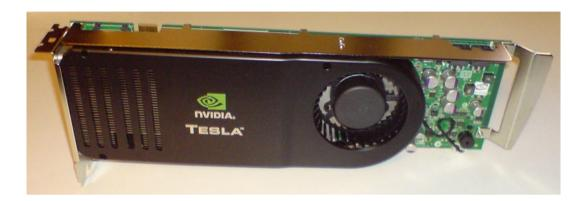
TESLA S1070 GPU 256 thread processors 1.5 GHz
