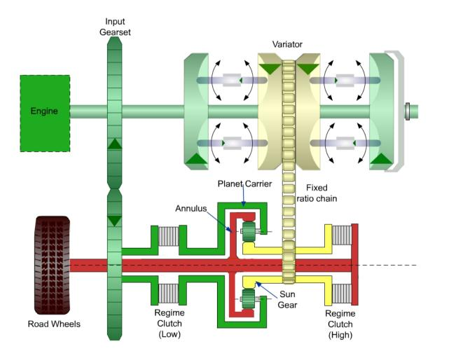
Torotrak use a "split path" layout with an epicyclic gear on the output side. This gives a geared neutral and hence infinite ratio and also a reverse, hence is an IVT.
