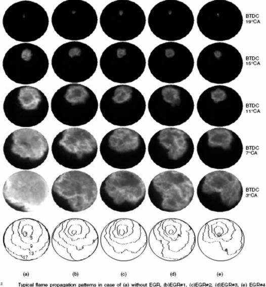
Typical flame propagation patterns in case of (a) without EGR, (b)EGR#1, (c)EGR#2, (d)EGR#3, (e) EGR# (number : crank angle after ignition (°CA))
