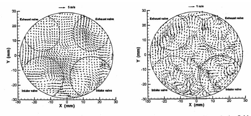
(e) Low-frequency fluctuating velocity field
