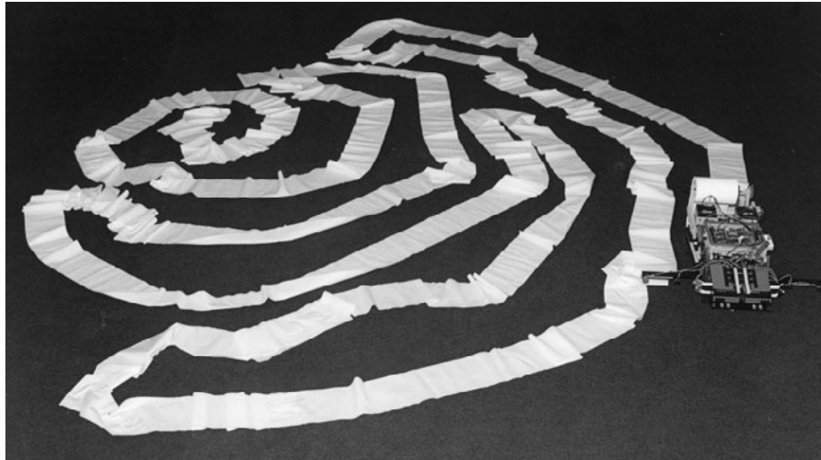
Figure 5 A robot meander. Control is passed from one side of the robot to the other every 30 s. As soon as control is swapped from one side to the other, the self-correcting nature of the thigmotaxis/phobotaxis reactions causes the robot to turn until contact is regained with the trail on the opposite side. Hence, the U-turn itself is not explicitly programmed. Note also the “starter spiral”, which is the result of “trail following” where there is no initial trail to follow. Similar starter spirals are seen in many meandering trace fossils. (Photograph from Prescott & Ibbotson, 1997.)
