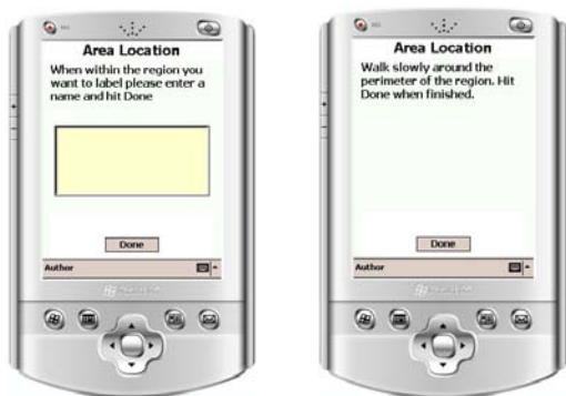
Figure 6: Defining location by walking a perimeter.
