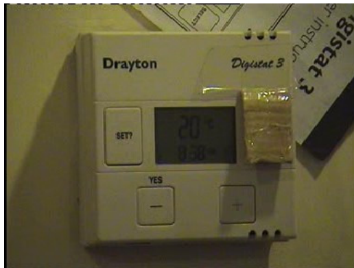
Fig. 1. Heating control modified using principles from aircraft cockpit design
