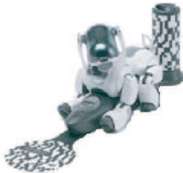
Figure 8: The AIBO recharging station target.
