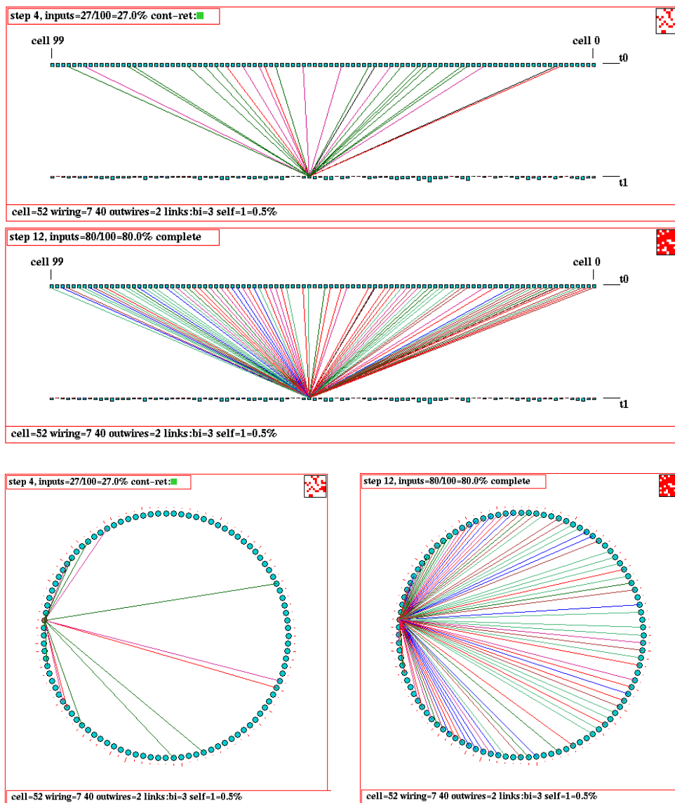
Figure 17.7: Recursive inputs (direct and indirect) to a given cell for a k=2 , n=100 RBN. Above: As time-steps. Below: As a circle. Firstly, inputs are shown after 4 backward steps with 27 cells reached. Secondly, the complete inputs are shown after 12 backward steps with 80 cells reached. A small 2d insert in the top right hand corner of the wiring window graphically indicates the fraction of cells connected so far.
