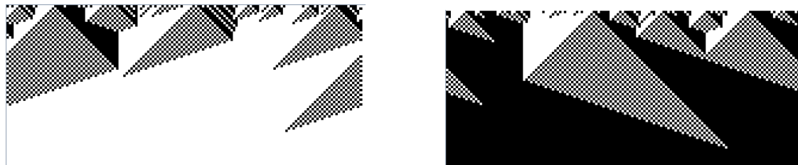
Figure 24.7: The density classification problem in emergent computation seeks to evolve a rule that is able to categorise states between a majority 0s and 1s. In this example of typical space-time patterns ( n=149 ), the rule is v2k7 (hex)(ff f0 8c f0 ff e0 00 f0 ff f0 00 f0 ef e0 00 e0), evolved by Raja Das[6].
