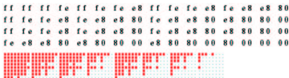
Figure 16.4: Setting the rule in hex. In this example the hex representation of the k=9 "majority rule" is shown, with its bit pattern representation below.
