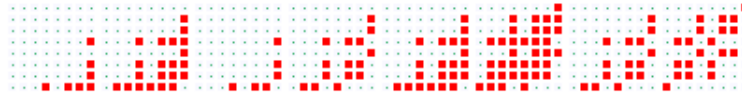
Figure 16.2: The game-of-life rule-table shown as a bit pattern. The 2^9 = 512 neighborhood outputs are ordered according to neighborhood value, with the all=1s neighborhood top-left and all=0s bottom-right.
