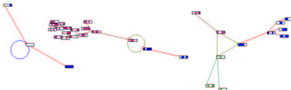
Figure 27.5: The basin of attraction field of an RBN, with states listed in section 27.7. n=5 , with mixed wiring k=3 , and a homogenous rule (dec) 110.
